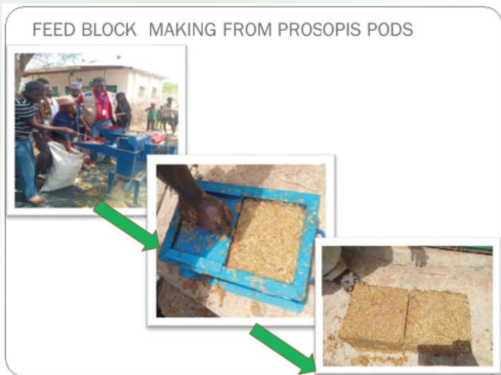
Figure 4 Prosopis juliflora feed block manual molding process
