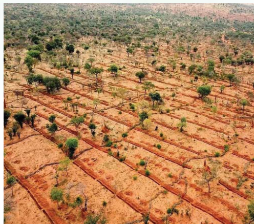
Plate 70: Water Retention ditches developed for reduced runoff and increased soil and water conservation for pasture establishment and rangeland rehabilitation
