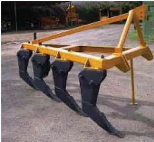
Plate 50: Tractor Chisel Plough for rainwater harvesting and creation of micro catchment and seeding lines for pasture
