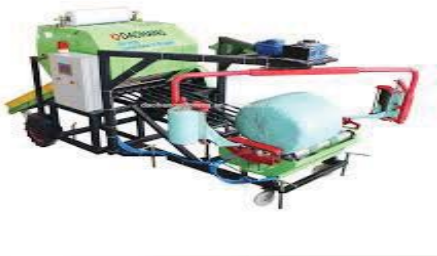
Plate: 145: Portable hay grass silage making equipment through airtight wrapping
