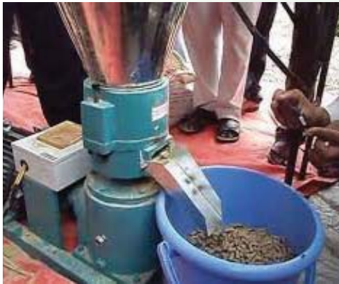
Plate 149: Pelletizer machine for small scale farmers
