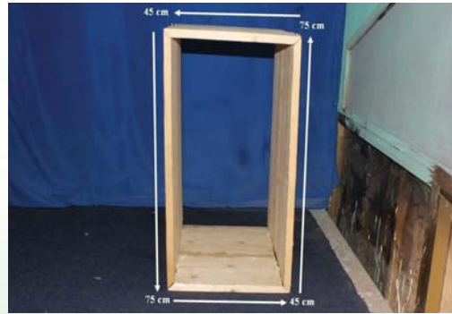
Plate 119: Hay boxes design and specification for standard hay making of about 17kgs
