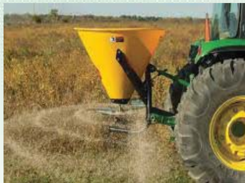
Plate 78: Tractor seed broadcaster for large scale production use. https://www.deere.com
