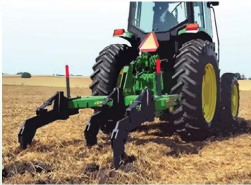
Plate 54: Tractor ripper from with three tines ripper
