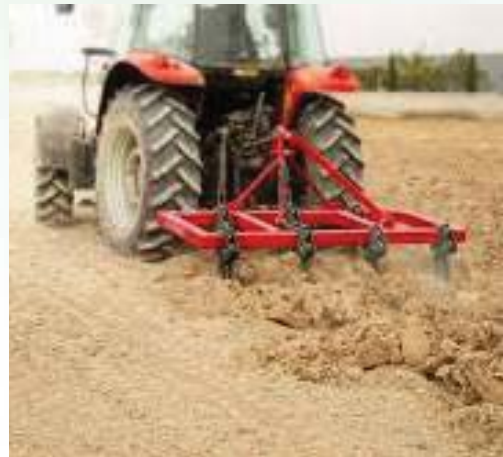
Plate 60: Chisel plough preparation of land for pasture reseeding
