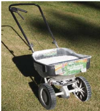
Plate 77: Hand-pushed broadcast spreader. Source: https://en.wikipedia.org/wiki/Broadcast_spreader
