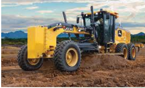
Plate 57 Grader plate used in contour terracing for reduced rub off and increased water infiltration
