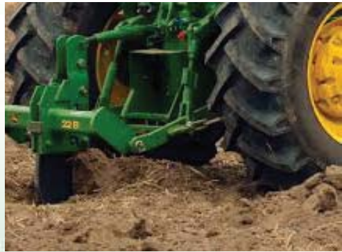
Plate 55: Tractor subsoiler for increased water infiltration/sinking water for rehabilitation and pasture establishment. Photos Source: https://kibbleeq.com/farmers/tillage/rippers
