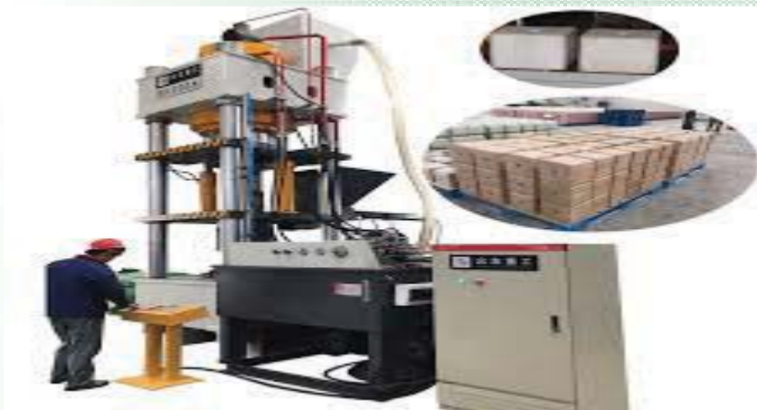
Plate 153: Hydraulic feed pelletizing machine for large scale commercial process. Photo source: https://china-hydraulicpress.en.made-in-china.com/product/KsinuclvLWhB/China-500t-800t-Animal-Feed-Block-Making-Hydraulic-Press-Machine.html
