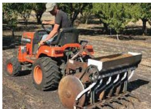
Plate 80: Mini tractor fabricated seed drill: Photos Source: https://farmhack.org/tools/home-built-no-till-seed-drill Sunny Slope Orchard o
