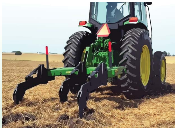
Plate 54: Tractor ripper from with three tines ripper
