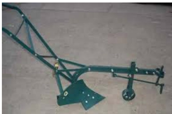
Plate 65: Animal drawn board plough for pasture-land preparation
