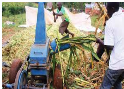
Plate 133: Tractor PTO silage chopper for silage making
