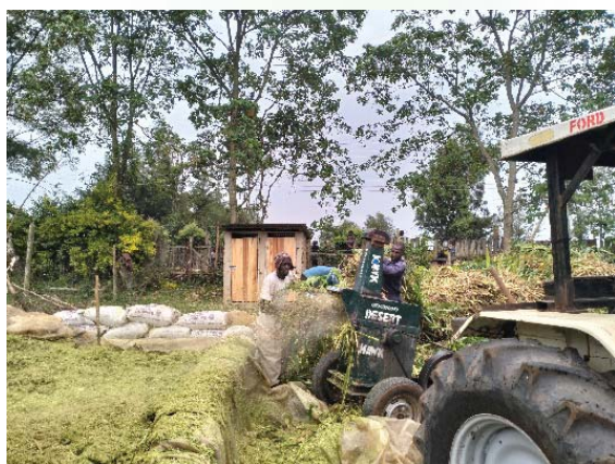
Plate 137: Tractor chopping silage with PTO driven chopper
