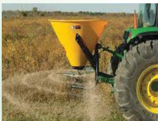
Plate 78: Tractor seed broadcaster for large scale production use. https://www.deere.com
